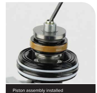
Piston assembly installed
